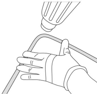
To form a curve or other shapes, place the seal on a heat-safe surface and gently warm the intend point of the curve with a hairdryer or similar, when the material becomes malleable simply bend it into the curve or other shape you require holding the hollowed side down.
