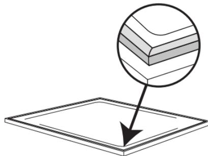
Measure out the length of threshold seal you require ensuring you will have a contact seal joint at each end. **DO NOT CUT THE SEAL UNTIL YOU ARE HAPPY IT IS THE CORRECT LENGTH.** If your intended area of application has a corner, this can be achieved either with a metred joint by cutting the threshold seal at 45 Degrees either side of the joint, or by forming a curve in the continuous length of the seal.
