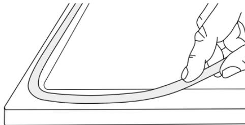
Carefully apply the seal with the adhesive attached to the intended area and gently press into place. The PVC crystal material is specially formulated to permit visibility through the seal to check that the adhesive has made sufficient contact with the surfaces, if gaps are visible, clean and repeat steps 3, 4, and 5.
