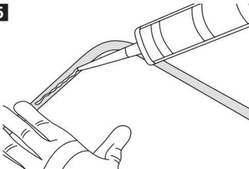
Carefully apply a minimum 7mm bead of neutral cure silicone adhesive to the centre of the hollowed side of the seal over its full length.
